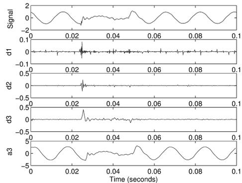
Fig. 3. Detail and approximation bands for a voltage dip signal taken from IEEE project group 1159.2, where the sampling rate is 15,360 Hz. The top plot corresponds to the original signal, and the detail bands are shown, from top to bottom, in increasing scale (decreasing frequency) order. The bottom plot corresponds to the approximation band of the coarsest scale.
