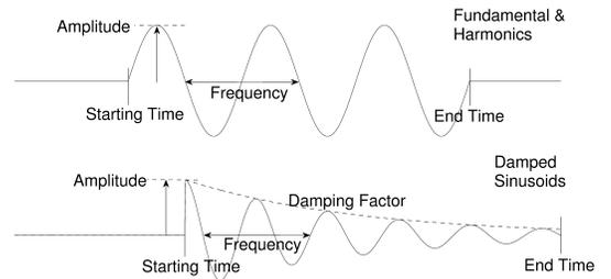
Fig. 5. Examples of parameterized atoms.
