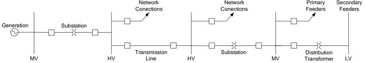
Fig. 1. A typical power system scheme (LV – low voltage, MV – medium voltage and HV – high voltage).
