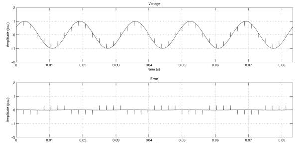
Fig. 4. Voltage signal corrupted by periodic transient events and residue obtained by subtracting the sinusoidal component.
