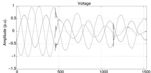
Fig. 2. A disturbance detected in a voltage signal measured in an MV electric circuit [65], showing transients and sags.
