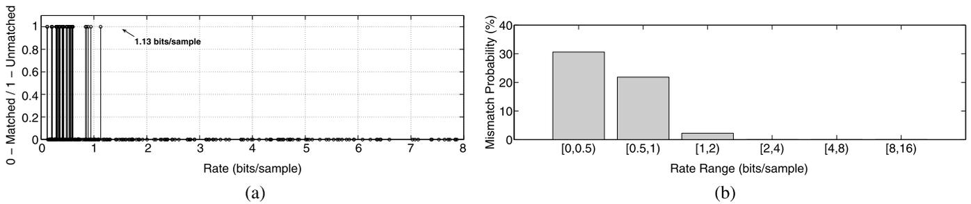
**Fig. 5.** Fault classification: (a) indicates which bit-rates values lead to classification mismatch and (b) shows the probability of fault classification mismatch for different bit-rate ranges.
