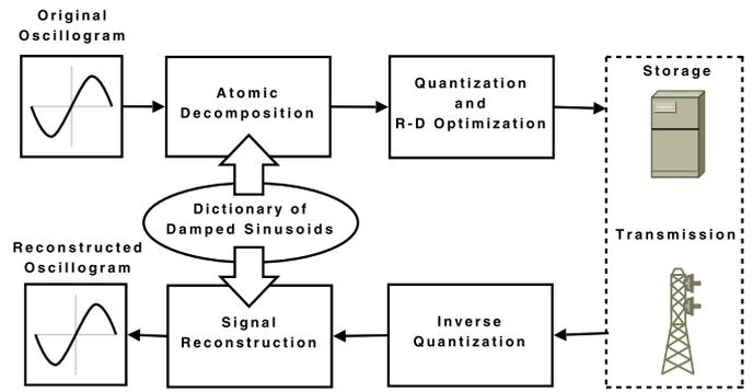
Fig. 2. General overview of the compression process of electric disturbance signals.
