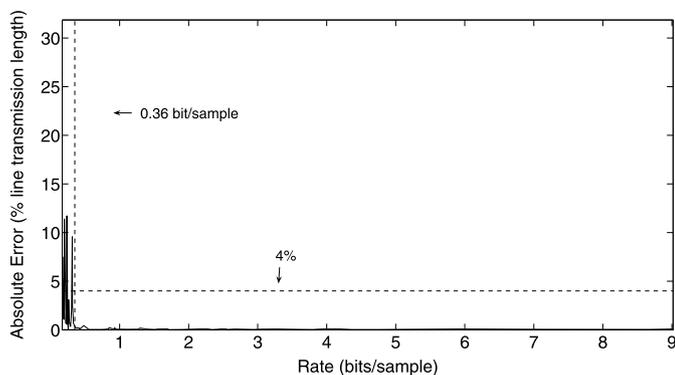
Fig. 7. Computation of fault distance modifying line conditions: absolute error versus bit-rate.
