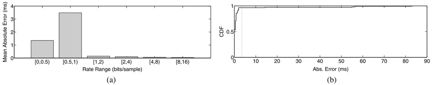
**Fig. 3.** Detection of the fault time instant: (a) mean absolute error versus bit-rate ranges, (b) CDF of the absolute errors of the fault time instant detection for bit-rates up to 1 bit/sample, the dashed line indicates 3.5 ms.
