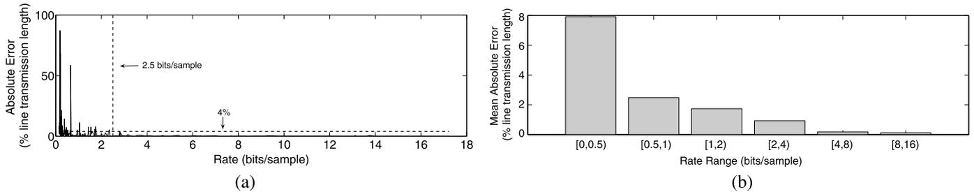
**Fig. 6.** Computation of fault distance: (a) absolute error versus bit-rate, (b) mean absolute error versus bit-rate ranges.
