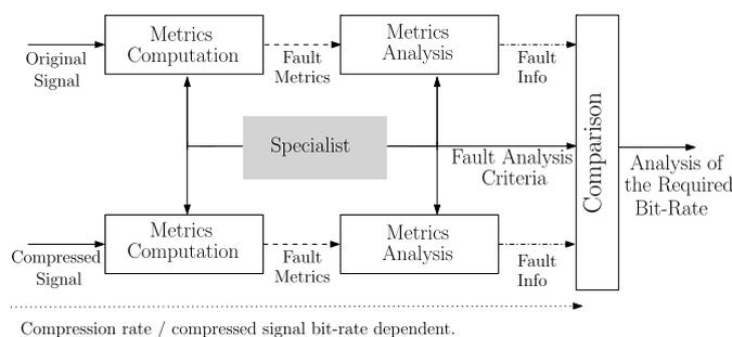
Fig. 1. Methodology employed for the assessment of the performance of the compression method.
