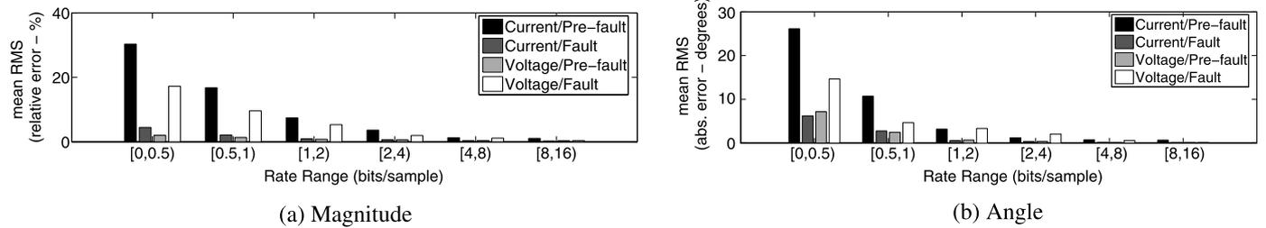
**Fig. 4.** Magnitude and angle computation of voltage and current in the pre-fault and fault periods: (a) mean RMS of relative errors of magnitude versus bit-rate ranges, (b) mean RMS of absolute errors of angle versus bit-rate ranges.
