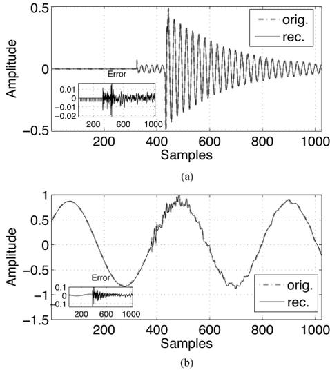
Fig. 5. Disturbance signals, their reconstructed versions, and errors at 0.95 and 0.578 bits/sample, respectively. (a) Signal  $R_1$ . (b) Signal  $R_2$ .
