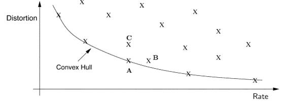
Fig. 4. Convex hull comprising the R-D optimal points.
