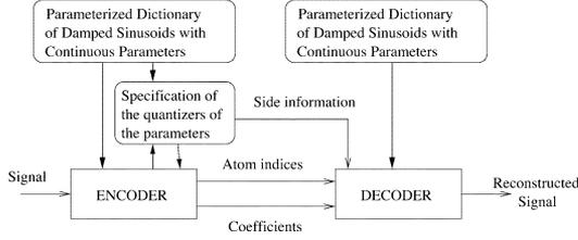
Fig. 2. Compression framework using a set of parameterized dictionaries.
