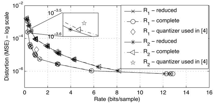
Fig. 6. Operational curves achieved by using the reduced and complete sets of quantizers for signals  $R_1$  and  $R_2$ .
