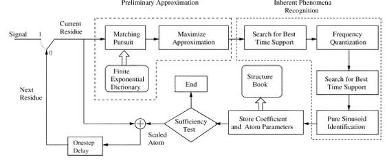
Fig. 3. Atomic decomposition algorithm. In the first iteration, the switch is in position 1 and in the remaining iterations stays in position 0.
