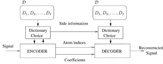
Fig. 1. Compression framework using a set  $\mathcal{D}$  of redundant dictionaries.
