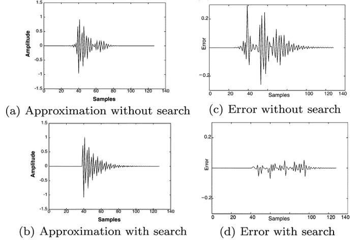
Fig. 3. Synthesis of synthetic signal  $SI$  [Fig. 2(a)] after decomposition using four steps of the MPs with densely sampled Gabor dictionary. (a) and (c) Without and (b) and (d) with the temporal support search of Section IV-B.
