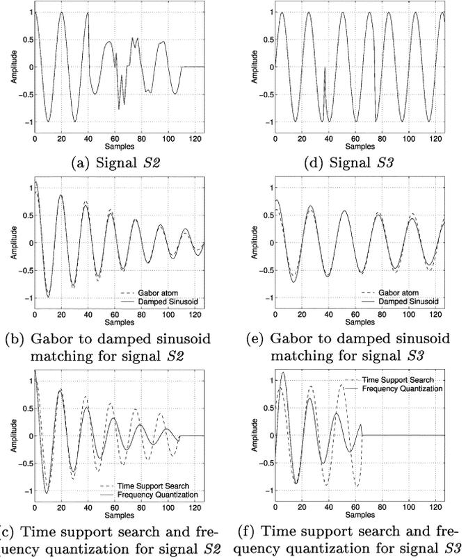
Fig. 4. First-step decomposition of synthetic signals  $S2$  and  $S3$  with time support search and frequency quantization.
