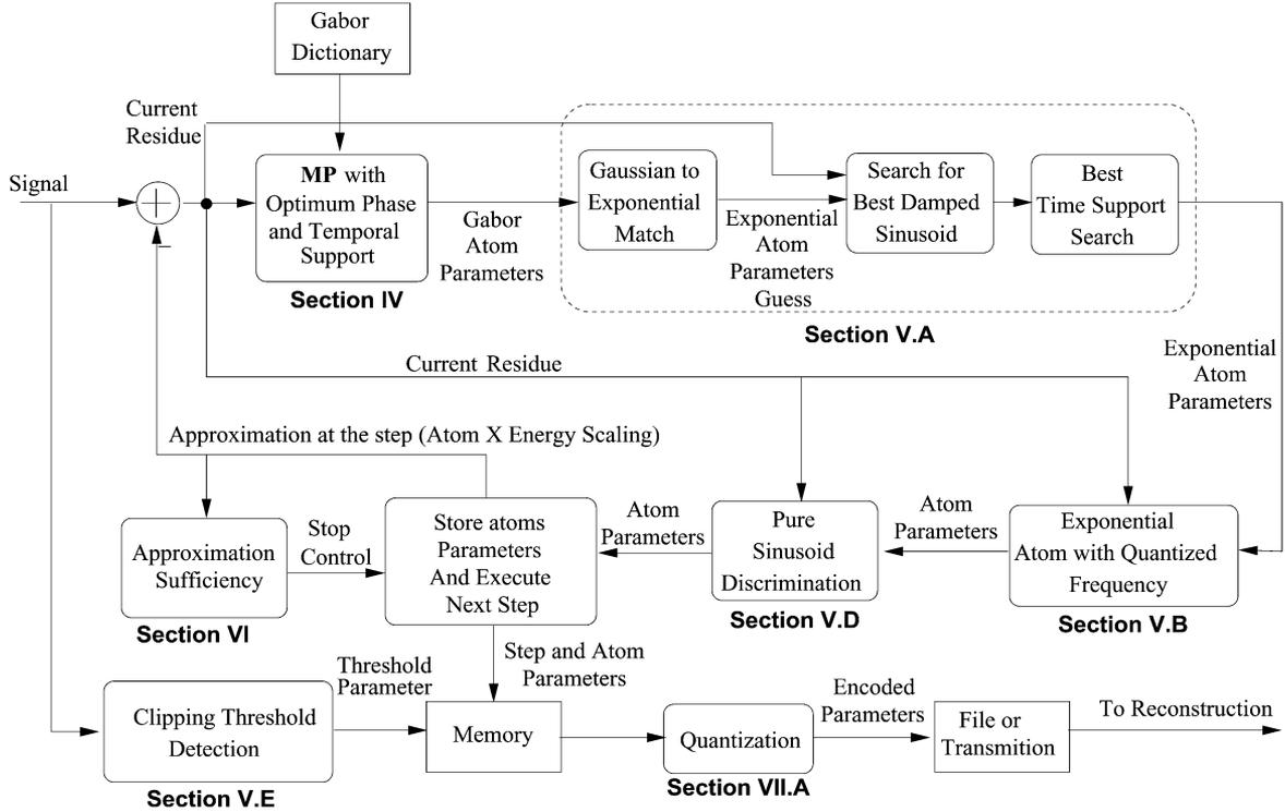
Fig. 1. Block diagram of the decomposition algorithm.
