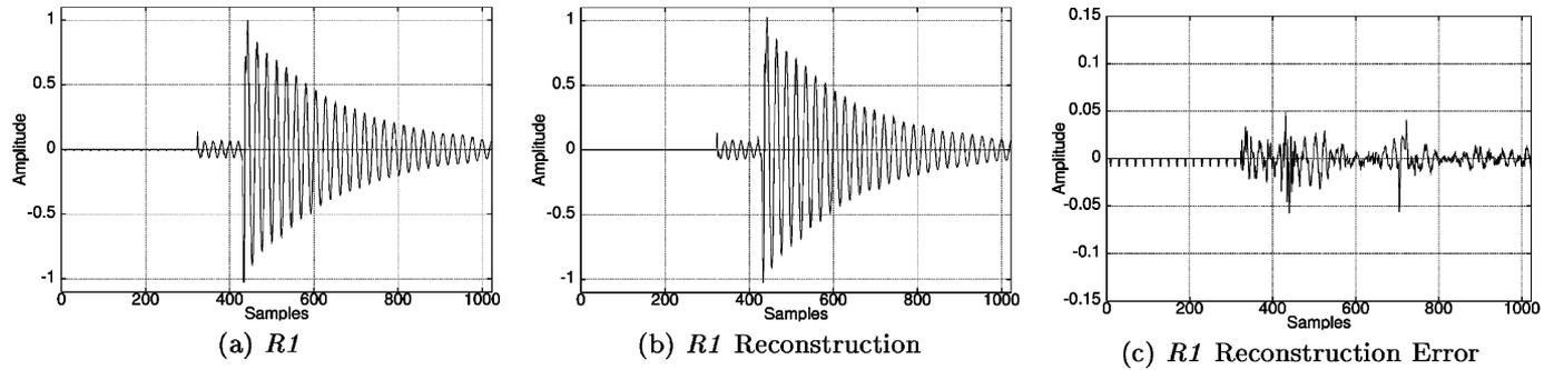
Fig. 10. Quantization of signal R1 with  $b_A = 6$ ,  $b_\rho = 7$ , and  $b_\phi = 7$ , where the compression ratio is 15.46, and the SNR is 28.08 dB at 1.035 b/sample.
