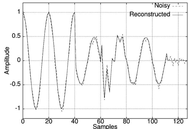
Fig. 9. Decomposition of synthetic signal S2 with noise addition in the damped sinusoid dictionary. The noisy signal is the dashed line, whereas the reconstructed one is in the continuous line.
