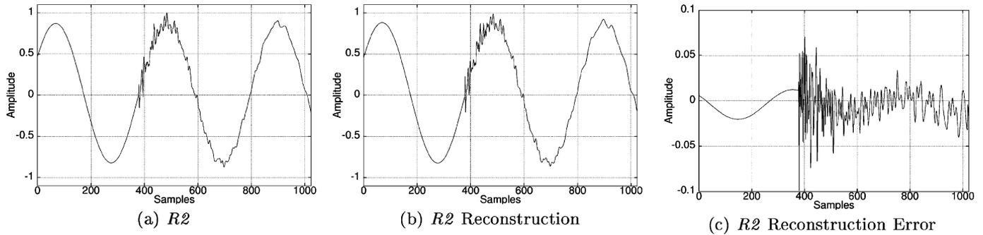
Fig. 11. Quantization of signal  $R2$  with  $b_A = 6$ ,  $b_\rho = 6$ , and  $b_\phi = 6$ , where the compression ratio is 27.40, and the SNR is 31.12 dB at 0.584 b/sample.
