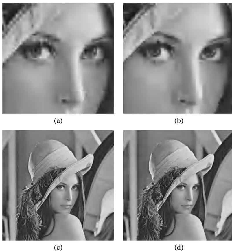
**Figure 4.** Lena image: (a) detail of face ( $128 \times 128$  pixel), coded at 0.15bpp using wavelets from filters A from [14] and (b) from the optimum filter of length 6/6; (c) Lena image coded with the 9/7 filter from [2] and (d) with filter F from [14] optimized for  $G_c \times PPR$ .
