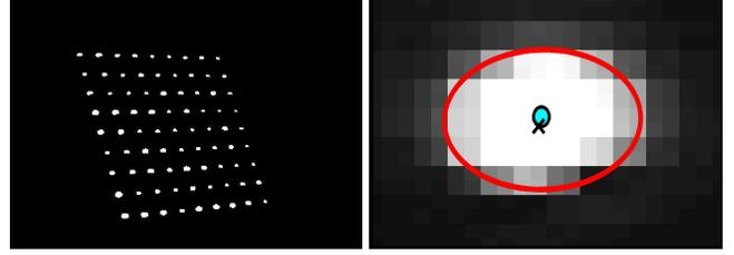
Fig. 3: Results of the calibration point localization. (Left) Fig. 1 after application of the thresholding operation. (Right) Zoomed version of Fig. 1 showing a single light bulb region with superimposed ellipse, and the obtained calibration point before (circle) and after (cross) the minimization of eq. (5).
