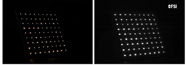
**Fig. 1:** Calibration device consisting of 81 light bulbs, arranged in a  $9 \times 9$  matrix, in the visible-light (left) and IR spectrum (right).
