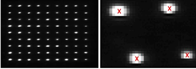
**Fig. 4:** Results of the iterative calibration point refinement. (Left) Undistorted equivalent of Fig. 1 in the fronto-parallel plane. (Right) Final calibration point positions for a few selected light bulb regions.
