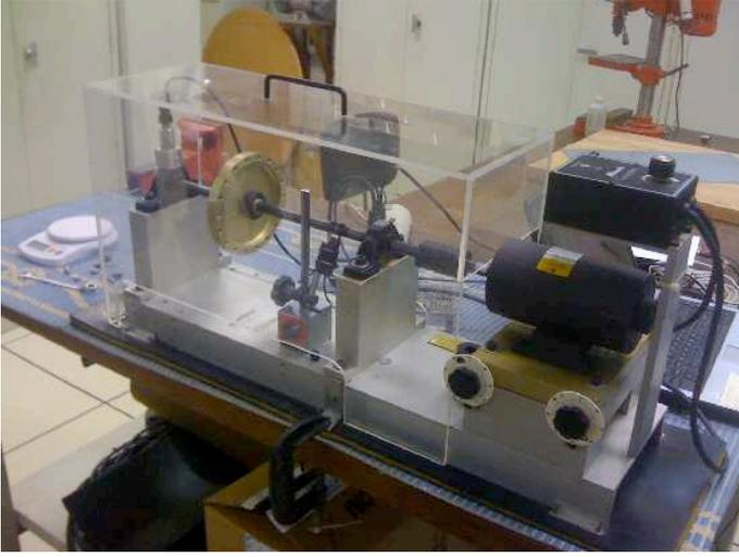
Fig. 1. Rotorkit used in the fault simulation scenario.
