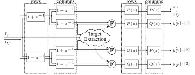
Fig. 4: Implementation of the 1<sup>st</sup> stage of the proposed fusion framework
