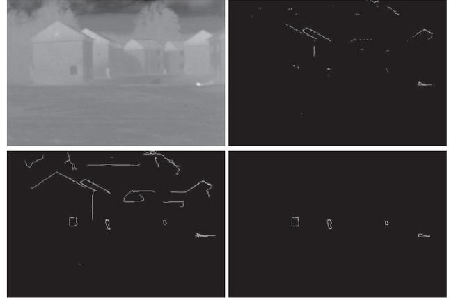
Fig. 2: Results of the target extraction. (Top-left) Original image. (Top-right) Seed points. (Bottom-left) Result of the tracking operation. (Bottom-right) Final result after application of the watershed transformation.
