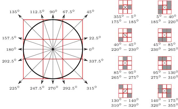
Fig. 3: Directional masks of the tracking operation
