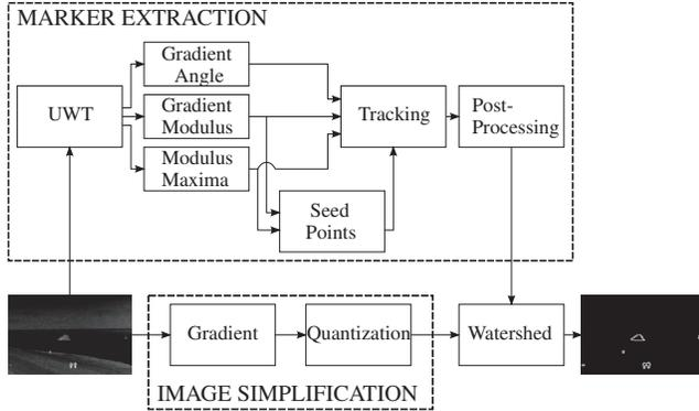
Fig. 1: Block diagram of the proposed target extraction approach
