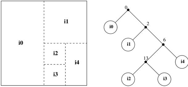
**Fig. 1.** Segmentation of a block and corresponding binary tree: the root corresponds to the original  $4 \times 4$  block (level 4), while nodes  $i_2$  and  $i_3$  ( $1 \times 1$  blocks) belong to level 0.
