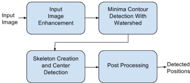
Fig. 2. Block diagram of the proposed method.
