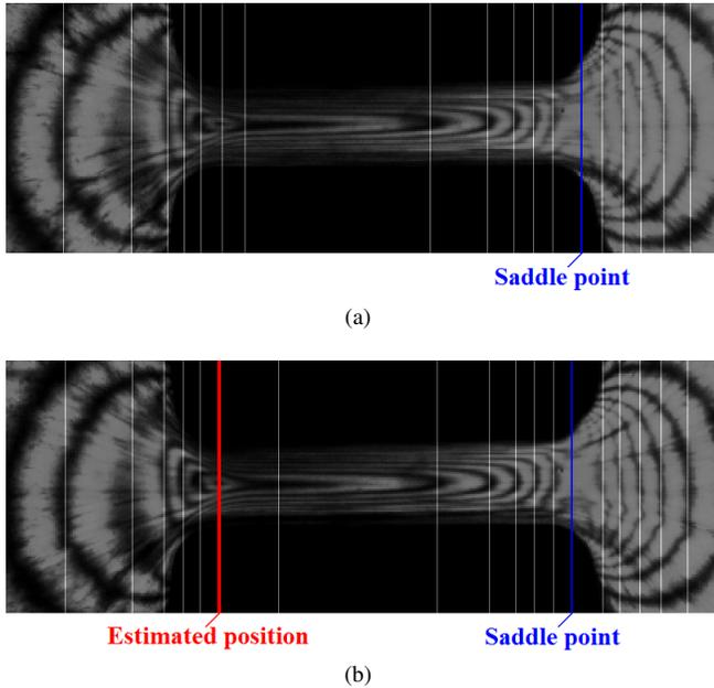
**Fig. 8.** Results of the algorithm for two birefringence images. The white lines represent the detected fringe positions, the blue line represents the saddle point and the red line is the estimated position when a fringe center could not be found.
