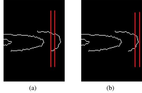
**Fig. 6.** Selection of points representing the center of the dark fringes. (a) Wrong selection — fewer segment points. (b) Right selection — most segment points.
